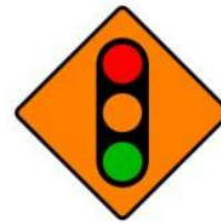
WK 060 - Temporary Traffic Signals
